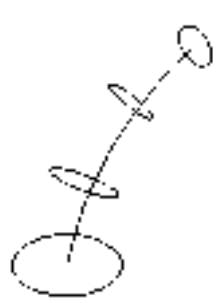
Cross Sections with Path curve
